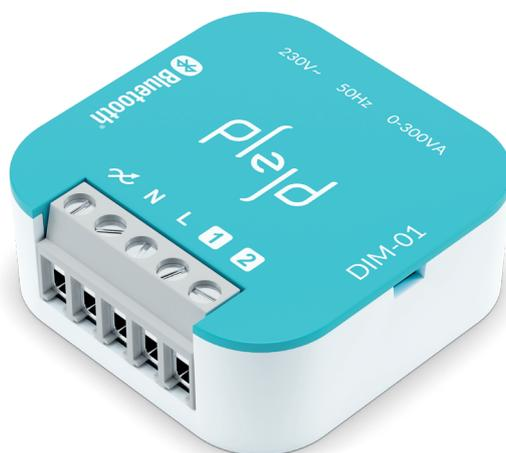
Universal dimmer with two separate inputs. The Dimmer LED can be controlled wirelessly via the app, via momentary push button or through other products from Plejd.
